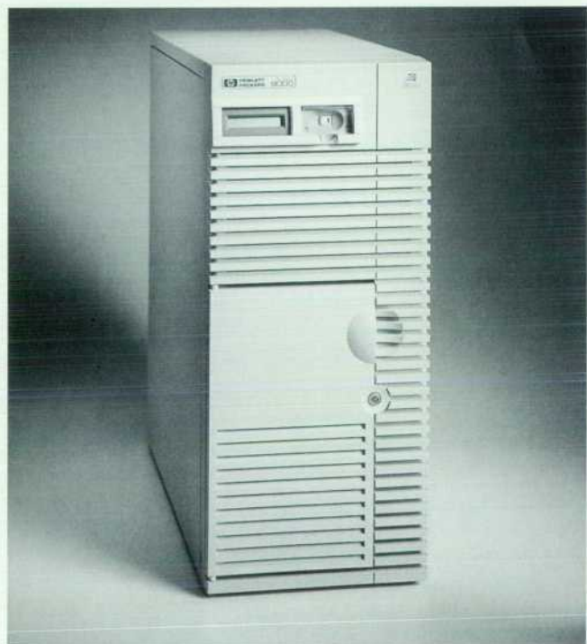
Fig. 1. The D-class server system cabinet. The dimensions of this cabinet are 10.2 in (26 cm) wide, 23.8 in (60.4 cm) high, and 22.2 in (56.4 cm) deep.
